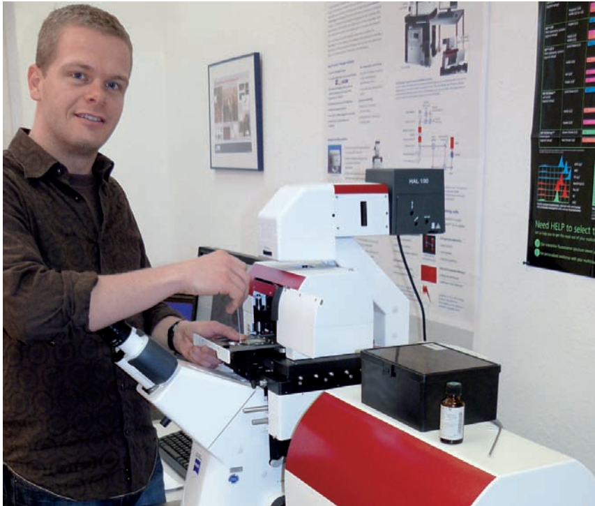
Figure 4: Dr. Joost van Mameren, application scientist at JPK: “We have integrated a piezo-based nanopositioning system into our NanoTracker to increase the accuracy and the experimental flexibility, e.g. to move at constant speed during an analysis.”
